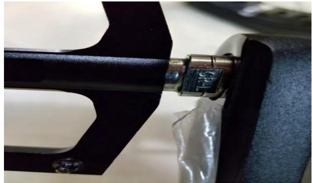
17. Attach right pedal by screwing into right crank in clockwise pattern using 15mm wrench (Note: recommend using a medium grade Loctite to ensure bolt does not loosen)
