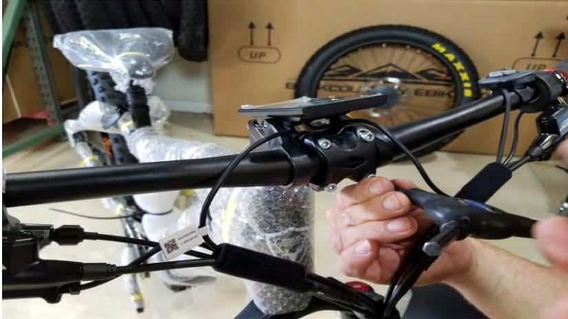
10. Display screen is easily rotated by hand forwards or backwards to customize to rider.
